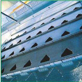
The system of air boxes allows the generated heated air to pass the entire length at a constant speed, and also increases fire safety. The variable cross-section of the boxes provides the same pressure of the heated air over the entire width of the dryer's shaft, thus ensuring high uniformity of grain drying.
