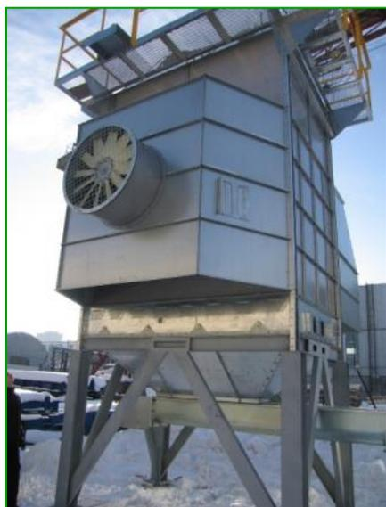
**1. Drier casing** is manufactured of anti-corrosion materials. The drier column comprises:
