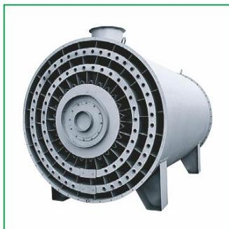
Air heater (burner) with a heat exchanger prevents carcinogenic combustion products from contacting the grain.
